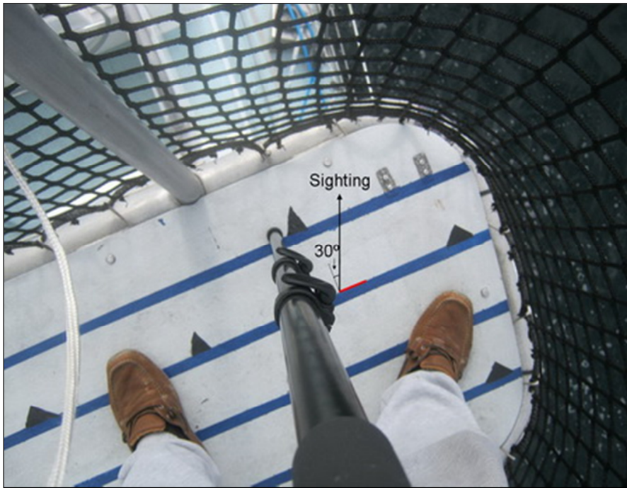
Figure 2: For every sighting from the observation platform a photograph was taken of the lines on the floor while the binoculars were pointing towards the sighting. Therefore an accurate calculation of the bearing to the sighting could be made from the angle of the lines on the A-frame in the photograph.
